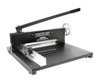
The 7000E is ideal for photo shops, schools, small print shops, and businesses. It cuts a full 12? length or depth and a stack of 1 1/2? of 20 lb. paper (approximately 350 sheets). The paper stop is adjustable and a positive clamp that holds paper in place, which eliminates shifting and tearing. A safety blade latch prevents cutting until it has been released. The precise English and Metric rule guides will aid in accurate cutting.
